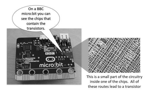
To give you an idea of size of these transistors, a human hair is approximately 80,000- 100,000 nanometres wide. In 2016, researchers at Berkeley Lab created a working transistor which is just 1 nanometre long.
